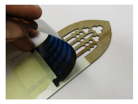
Next remove the masking tape and lift that side up, remove the protective tape covering and press the film down into the adhesive. This approach will ensure you get the glass aligned with the window openings properly. (see photo on following page).
