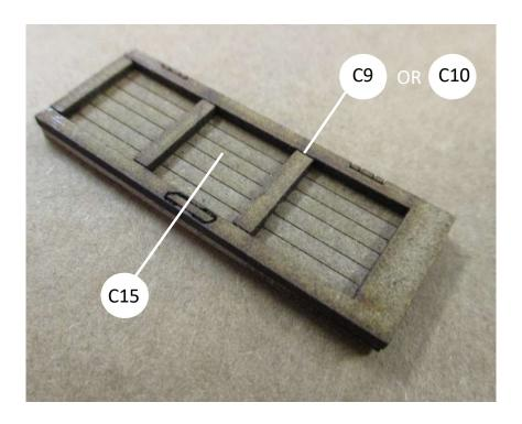
**Step 17**: There are two separate doors, in the event you choose to position them open. For the manual we chose to keep them closed. In either event the doors need to be glued into position inside the door frame, as shown below.
